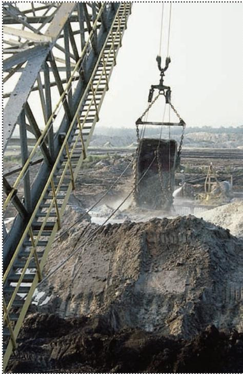
Figure 8. The dragline bucket is large enough to hold a car. It weighs 110,000 pounds and is secured by ten 4-inch thick steel chains.
